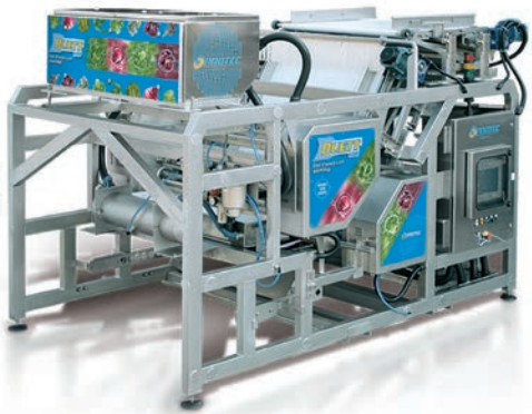
Air ejection sorter with 2 or 4 vision cameras system for fresh vegetables, fresh-cut and fruit dices. Inspects the product on both sides.
